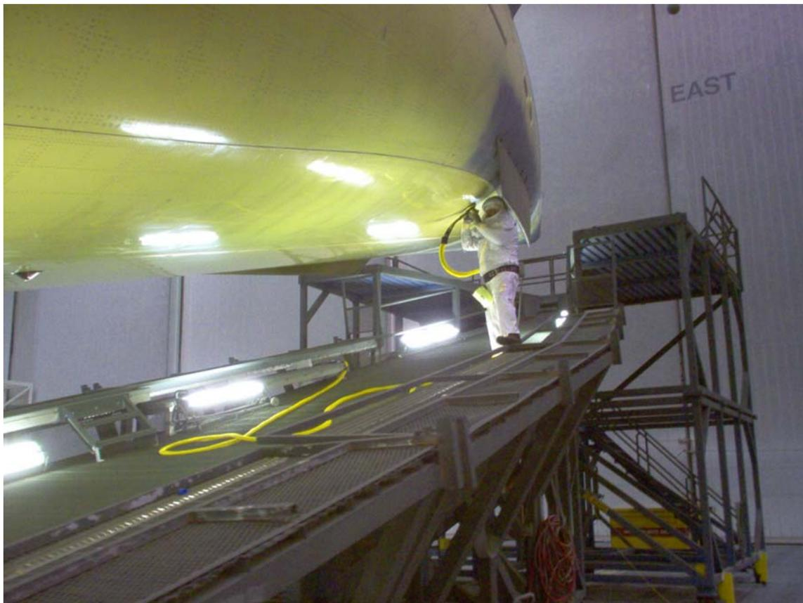
**Technician on tail ramp attached to vacuum line on tail ramp using hose support Belt**
