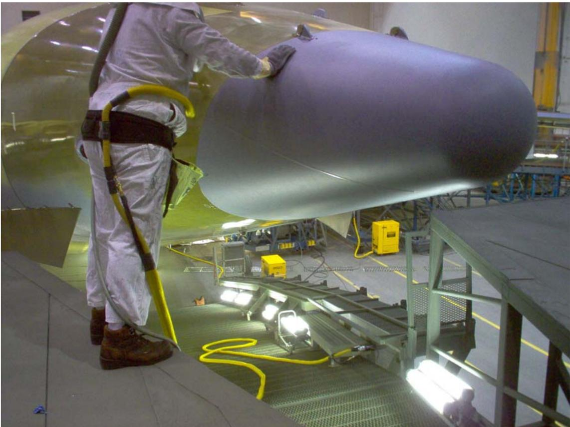
**Technician on tail attached to vacuum line on tail ramp using hose support belt**
